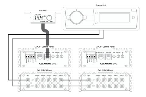
The ZVL can be simultaneously used as a master volume controller and preamp for multiple sub amps, and an active full range signal RCA distribution block.
