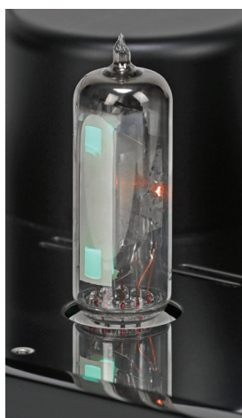
An EM84 valve shows music level in a light blue fluorescent display that's entertaining – especially in the dark.
