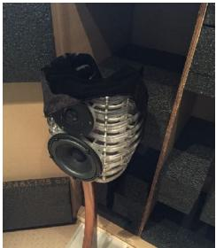
Remove the bass module by pulling carefully on its acrylic base. The bass module is heavy and might require a second person to pull it out.
