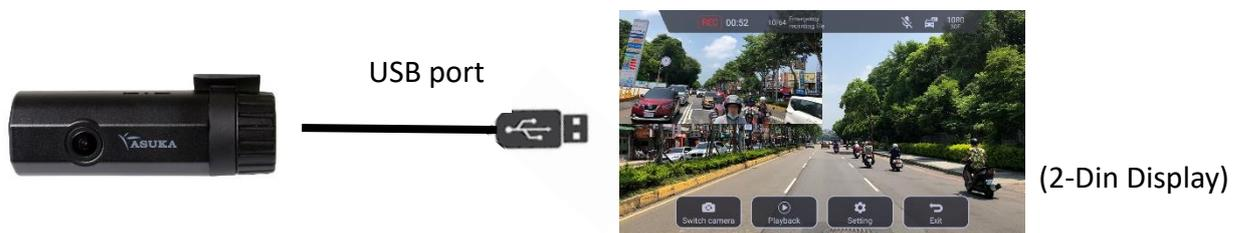
The USB connector contains wiring for powering, video signal, and command control. So, no additional wiring is required.
